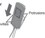
② Insert the controller until the two protrusions on the controller holder click into the cavities on both sides of the controller.
