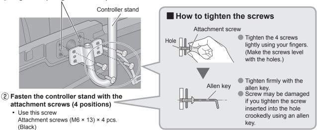
If the controller stand is attached on the left hand side, pass the controller cord through the left hand side. (Page EN17)
