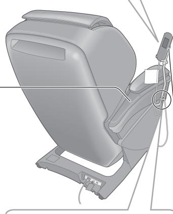
Fasten the controller cord using the cord clip. Fasten so the cable under the cord clip will not sag too much (because of the risk of tripping over the cord).
