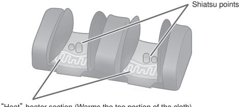
"Heat" heater section (Warms the toe portion of the cloth)
